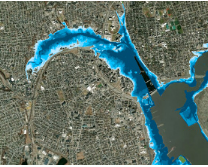
Current flooding possibilities from a 1% annual chance storm with level darkness linked to water height. At the darkest places it is more than 11 feet. Maps made by author in Stormtools.
